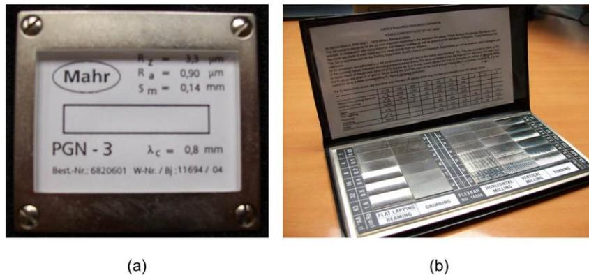
Figure 5 – (a) The Mahr™ standard and (b) the Flexbar™ standards.
