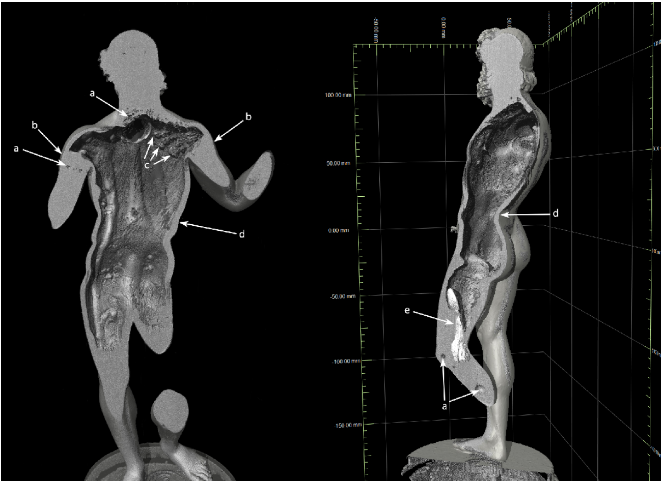
Figure 2. X Tomography of Jupiter statuette, with two virtual sectional plans. (images Elsa Lambert et Jérôme Rumolo , C2RMF). Those images show a) numerous porosity, b) location of welding, c) infiltration of welding metal d) thickness of wall, e) secondary cast of fettling (an alloy of lead and tin)
